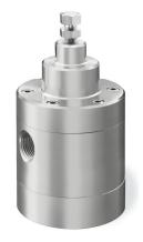
TESCOM 26-2900 Series is a dome loaded, negative bias, backpressure tracking regulator with a balanced main valve. This regulator controls upstream pressures up to 1000 psig / 69.0 bar with spring bias setting.
